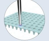
Single well detector-based (non-fiber optic) systems must move 96 times to read each channel.
