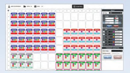
Quickly set up and confirm plate layout. Each well is color coded by sample type, biological replicate, and technical replicate. Well type and standard curve values are also easily visible.
