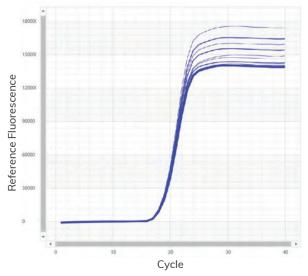
Optical design eliminates need for ROX. Amplification curves generated using human genomic DNA template along with human GAPDH primers and a no ROX SYBR Green qPCR mix.
