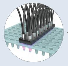
The Azure Cielo 6 Real-Time PCR system moves 6 times in 9 seconds to scan an entire 96-well plate.
