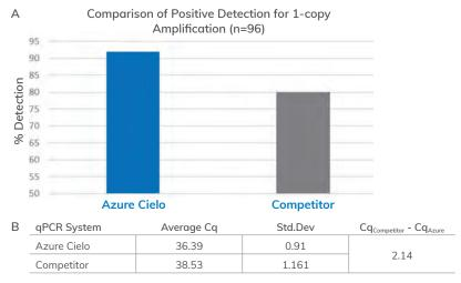
Superior single copy detection. Real-Time PCR was carried out using BioRad Prime PCR Probe Assay for GAPDH, 1 copy of Human Reference GAPDH DNA Template and Biorad Multiplex Supermix. A) Comparison of amplification detection in Azure Cielo Real-Time PCR system and Competitor shows higher rate of 1-copy detections. B) Average Cq obtained from Azure Cielo System is 2 cycles earlier than Competitor. Cqs from the above experiment were averaged.
