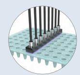
8 well channel systems have to move the scan head 12 times to read each channel.
