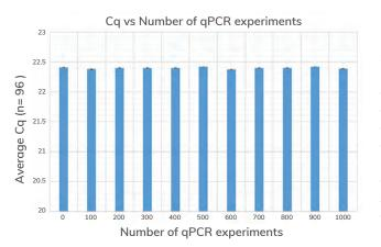
Robust design. After sequential sets of 1000 continuous qPCR experiments, a GAPDH qPCR assay was performed and Cq values were recorded at every 100 experiments points. Average Cq in each assay = 22.4, ±0.01.
