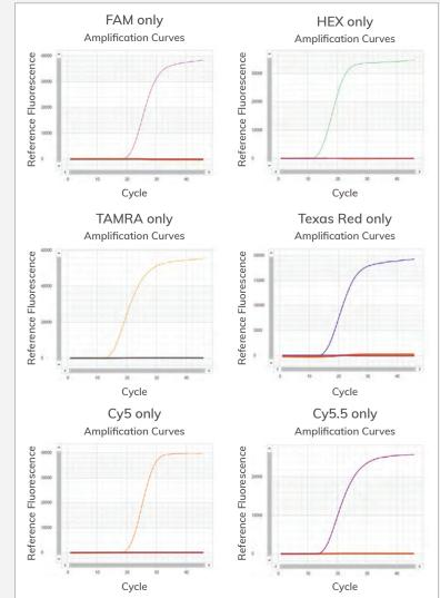
Multiplex qPCR reaction were scanned for all 6 channels in an Azure Cielo Real-Time PCR system. Single channel amplification curves were as expected, with no signal leakage or crosstalk.
