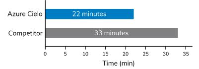
A commercially available fast qPCR kit was run, using SYBR Green. Protocol as follows: 95°C, 2 minutes, 40 X (95°C 1 second, 60°C 1 second).
