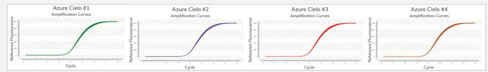
Reproducible data on four separate Azure Cielo instruments using Human GAPDH assay and SYBR Green Master Mix. Average Cq = 20.11, SD= 0.002
