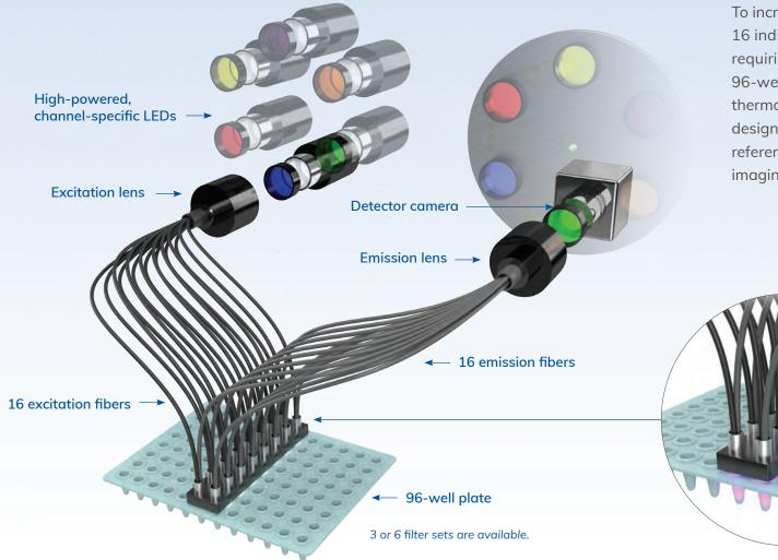
To increase speed, Azure Cielo images 16 individual wells simultaneously, requiring just 6 scans to scan an entire 96-well plate. Combined with high thermal block uniformity, Azure Cielo's design avoids the need for a passive reference dye and enables faster imaging times.
