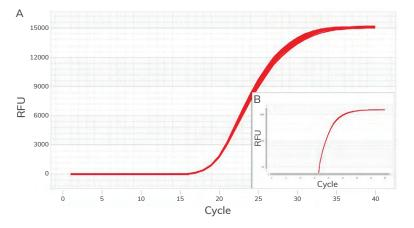
Unparalleled uniformity. Amplification curves for 96 replicates shown on a linear plot (A) and a logarithmic plot (Figure B). In each well,  $10^5$  copies of GAPDH template were amplified in the presence of GAPDH primers and BioRad<sup>™</sup> Sso Advanced SYBR Green Mix<sup>®</sup>. Average Cq = 19.1, Coefficient of variance (Cv)= 0.002.
